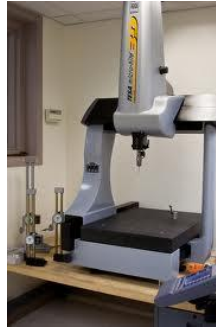
Fig. (2) A 3-Axis coordinate measuring machine
