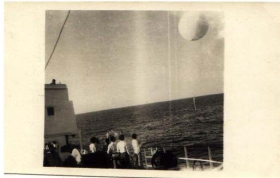
Fig. (3) A weather sounding balloon being launched from a research vessel (Ship)
