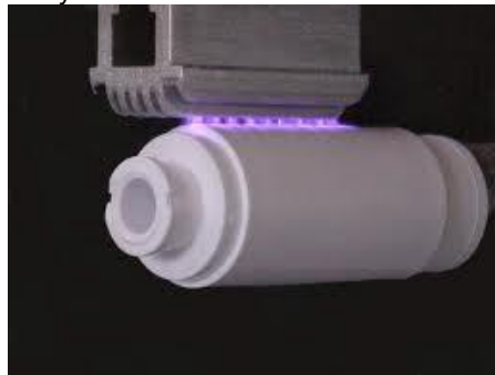
Fig. (1) A High Voltage Corona discharge Treater in operation
